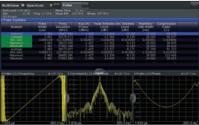
▲ Fig. 2 LFM compressed pulse. The correlated magnitude window shows the peak sidelobes are approximately 13 dB down from the peak.
