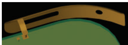
▲ Fig. 1 Unmatched GPS-Bluetooth antenna.
