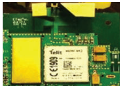
▲ Fig. 6 Assembled prototype of the hybrid antenna.
