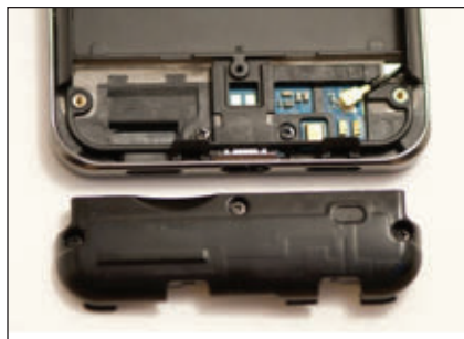
▲ Fig. 2 Antenna integrated into the package. 2
